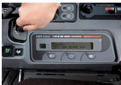
2 Insert new individual Black operational key.
