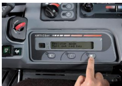
1 Insert the Red programming key, then press the monitor button.
